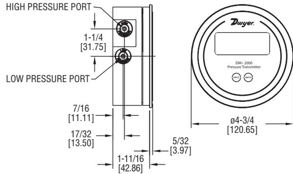
The Dwyer **SERIES DM-2000** Differential Pressure Transmitter senses the pressure of air and compatible gases and sends a standard 4-20 mA output signal. The DM-2000 housing is specifically designed to mount in the same diameter cutout as a standard Magnehelic® gage. A wide range of models are available factory calibrated to specific ranges.
